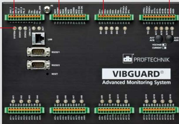
16 analog measurement channels for vibration signals
