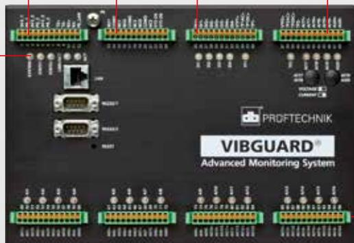
16 analog measurement channels for vibration signals
