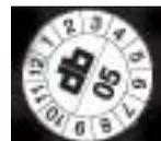
The calibration label is affixed on the back of INCLINEO and shows the date of the next scheduled calibration.
