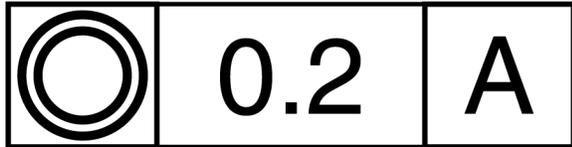
Concentricity measures how well a cylinder (line) fits inside of another cylinder (line).
