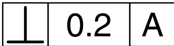
Perpendicularity measures the condition of a plane at a right angle (90 degrees) to a datum plane.
