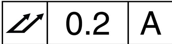
Total Runout controls the composite surface variations of circularity, cylindricity, parallelism, straightness, taper and profile of a surface where applied to features constructed around a datum axis. Total Runout applies to an entire surface simultaneously, not just individual circular elements.
