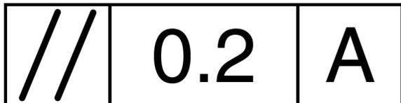
Parallelism measures the condition of a plane that is equal in distance at all points from the datum plane.
