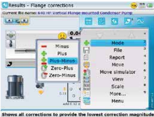
Shows all corrections to provide the lowest correction magnitude.
